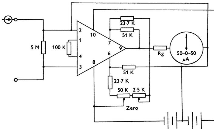
Fig. 1. Circuit for current measurement. The amplifier is a Burr-Brown 3670J used at unity gain. Output of the amplifier is 5 mV/nA and  $R_g$  is selected according to the range of currents which are to be measured. Rechargeable batteries providing  $\pm 7$  to  $\pm 20$  V may be used.
