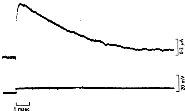
Fig. 1. 'Capacitive' current due to a 5 mV depolarizing step. The finite peak of the current is due to the presence of a significant resistance in series with the membrane. The slow rise is probably due to the presence of a small stray capacitance. The capacitive current decays exponentially, the average time constant being 4.9 msec. The steady-state current reflects the sum of the series resistance and the membrane resistance. See text for further details.
