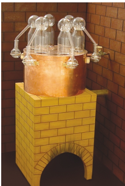
Apparatus for distilling rose water. Replica built by the Institute for the History of Arab–Islamic Sciences, according to a description by the physician az-Zahrāwī from the late tenth century in Muslim Spain. Image courtesy of Fuat Sezgin, Institute for the History of Arab–Islamic Sciences, University of Frankfurt, Germany.
