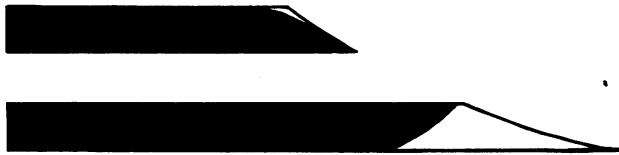
Fig. 1.—Cross-section of needle, as manufactured and as ground down for intracorneal injection.
