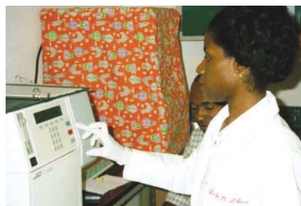
Fig. 3 | FACS (flow cytometer) machine at the Clinique Bon Sauveur, to perform CD4 counts for rural HIV patients. © 2002 Partners in Health.
