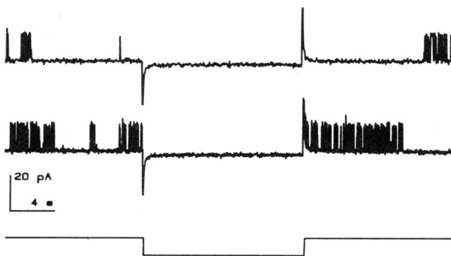
FIGURE 3 Ba^{++} trapping experiment. A channel was exposed to 1.9 \mu M internal Ba^{++} at a holding potential of 45 mV, and the voltage pulse protocol was applied as described in the text. Upper trace: a 15-s hyperpolarizing test pulse to -70 mV was applied during a blocked interval. The computer recognized a blocking event as a nonconducting state lasting for longer than 800 ms. Under these conditions, the average block time is 3 s, while the average closed time is 2 ms; the identification of the blocked state is therefore unequivocal. Lower trace: a similar pulse applied during a burst, when the channel is not blocked. To identify whether the channel is blocked or unblocked after the test pulse, the channel record is examined immediately after returning to 45 mV; if the channel fails to open during the first 200 ms after returning to 45 mV, the channel is scored as being blocked. In this example, the first latency to opening was 11 s in the upper trace, and <10 ms in the lower trace.
