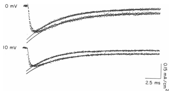
FIGURE 7 Superimposed I_{Na} records at the two potentials indicated. These records are the first 20 ms of those from the right hand column of Fig. 1 shown on a somewhat expanded time scale. Superimposed on each of the four records is a single exponential fit to the inactivation time course ( thin lines ; extended to the start of the potential step). Fits were generated with the aid of the PDP 11/34 using a nonlinear least squares procedure. During the inactivation phase, the fitted exponentials are not distinguishable from the current records. Fitted \tau_h values are 5.38 ms in K_i and 5.49 ms in Cs_i at 0 mV, and 4.42 ms in K_i and 4.78 ms in Cs_i at 10 mV.
