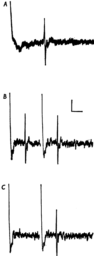
Fig. 1. A , photograph of three oscilloscope sweeps superimposed to show the constant latency of the antidromic action potential, the initial deflexion is a large stimulus artifact and the second is the antidromic potential. B , a train of two pulses each followed by an antidromic action potential. C , the same train of two impulses triggered by a spontaneous action potential. In this case the first antidromic action potential collides with the spontaneous spike and disappears but the second appears as expected (scale mark: A , 0.2 mV and 5 msec; B and C , 0.2 mV and 10 msec).
