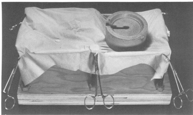
FIG. 1. Twin sling experimental setup with suspension of Serratia Marcesens 10.6 ml. in water in each hammock. A 2 kilogram weight is placed in one hammock while the other serves as a pressure-free control.
