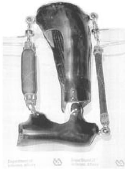
Figure 1. Powered ankle-foot orthosis. The carbon fiber shell has an artificial pneumatic dorsiflexor (maximally inflated) and artificial pneumatic plantar flexor (relaxed) attached via titanium fittings.
