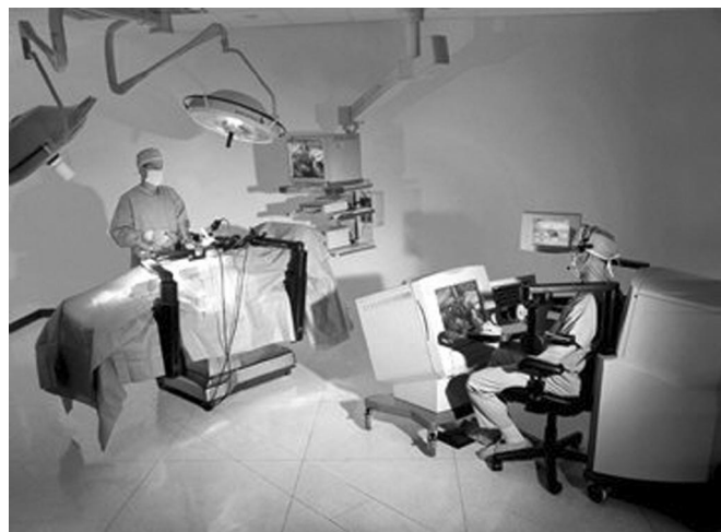
FIGURE 2. Zeus system set up. (Courtesy of Computer Motion Inc., Santa Barbara, CA)
