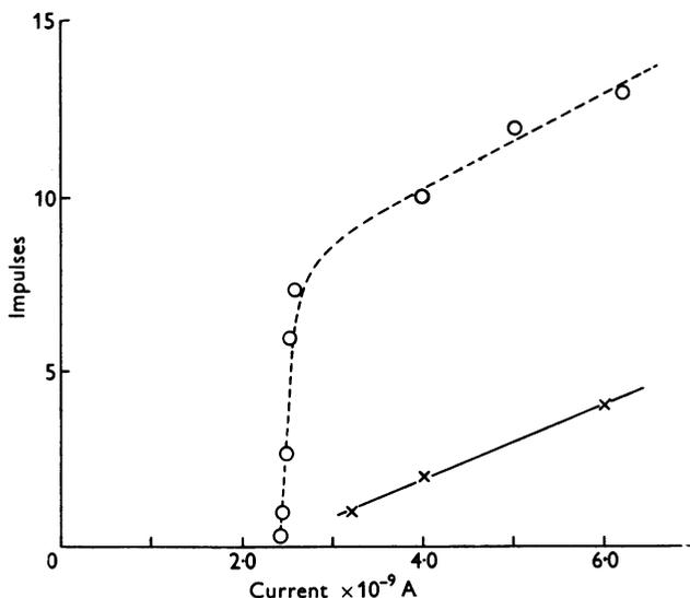
Fig. 8. Repetitive response of a motor axon (—) and interneurone soma (---) to current pulses of 14 msec duration. Rheobasic current: for interneurone soma  $1.5 \times 10^{-9}$  A, for motor axon not known accurately but approximately the same.
