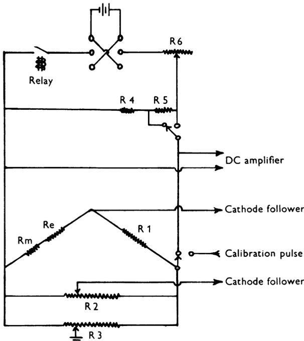
Fig. 1. Schematic view of recording and stimulating circuit.  $R_1 = 500 \text{ M}\Omega$ ,  $R_2 = 10 \text{ k}\Omega$ ,  $R_3 = 10 \text{ k}\Omega$ ,  $R_4 = 100 \Omega$ ,  $R_5 = 1000 \Omega$ ,  $R_6 = 10 \text{ k}\Omega$ ,  $R_e$  = electrode resistance,  $R_m$  = membrane resistance. Relay is Clare mercury wetted type.
