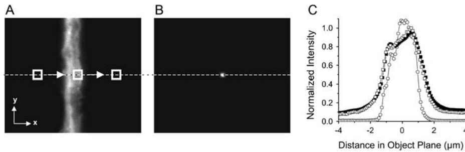
This scaling factor calibrates the counts on the 16-bit scale of the camera into photon counts measured by the APD. Notice that the two curves collapse onto each other, indicating that the window function used in the convolution is accurate. The same dendrite is then illuminated with the laser spot, and the image is scanned across the same pinhole and APD as above (○). This is scaled to best match the scan using the APD and arc lamp. This scaling factor provides the calibration of the lamp intensity in terms of the laser intensity.
