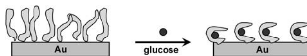
FIGURE 11 A schematic of spatial organization of GGRQ26C proteins before and after adding glucose.
