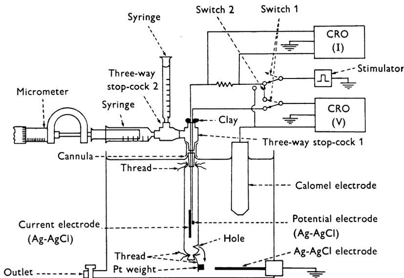
Fig. 1. Diagram of the arrangement for internal perfusion. For stimulation and recording of action potentials, switch 1 is set as shown in the lower position (solid). For measurement of resting potentials, switch 1 is set in the upper position (interrupted); the base line of the pre-amplifier may be checked by short-circuiting its input by means of switch 2.
