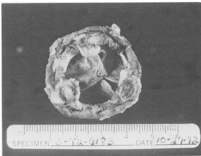
FIG. 3. Locally mounted valve with failure and replacement at 42 mos. The leaflets are thin and pliable but all three commissural attachments have pulled off posts (Leaflet tears were done at removal).
