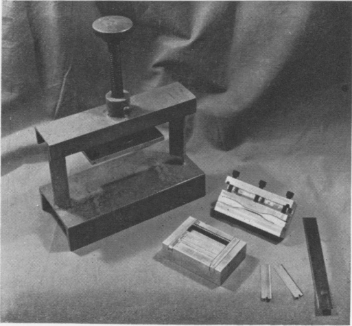
FIG. 3. Cutters used to prepare specimens for testing. Die at left is for wounded specimens while the one at right is for unwounded specimens.
