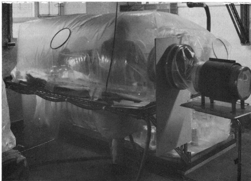
Fig. 2 A large flexible film isolator used to rear calves. The half-suit worn by the attendant in the foreground protects him from direct contact with the interior of the isolator without interfering with his manipulations. A steam-sterilized drum is shown attached to the entry port on the extreme right.
