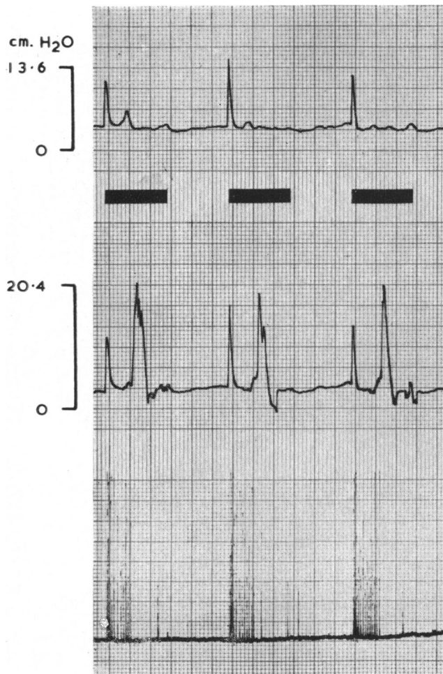
FIG. 2. Tracing of pressure and flow in a rat preparation. Upper tracing, pressure in body of stomach; middle tracing, pressure in antrum; lower tracing, flow record, each vertical stroke corresponding to one drop. One-minute periods of stimulation indicated by black bars. Note that peristalsis and flow occurred only during periods of stimulation.
