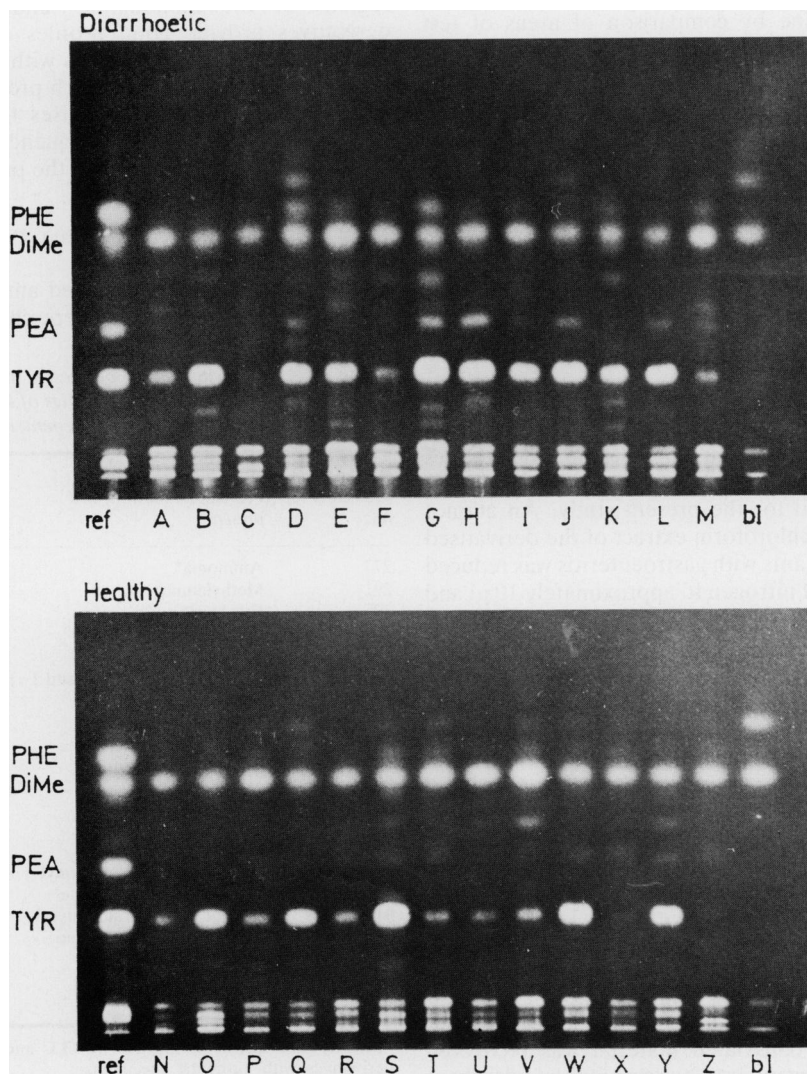
Fig. 2 One dimensional thin layer chromatograms of dansylated faecal amines and phenol of diarrhoeic and healthy infants. PHE=phenol, PEA=2-phenylethylamine, Tyr=p-tyramine, DiMe=dimethylamine (from reagent).
