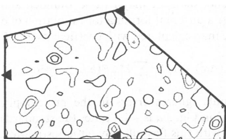
FIGURE 4 120° sector of a test map calculated with amplitudes |F_{N1}| - |F_{N2}| , where F_{N1} and F_{N2} are derived from two different subsets of the native bR electron diffraction patterns. The contour interval is the same as for Fig. 3 a.
