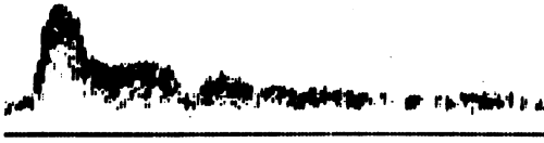
Figure 1. Directional common carotid sonagram over one cardiac cycle from a healthy young volunteer, showing Doppler-shift frequency on the ordinate and time on the abscissa. Blood flow towards the brain is displayed above the horizontal line and any reverse flow is displayed below the line. The blackness of the trace at each point is related to the number of erythrocytes generating the same frequency, i.e. moving at the same velocity. Two peaks are present during cardiac systole and no reverse blood flow is shown
