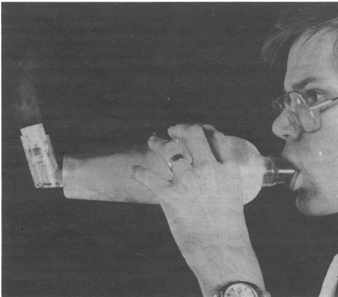
Simulation with solid CO 2 of subject with low flow rate failing to close valve on expiration and blowing aerosol out of reservoir.
