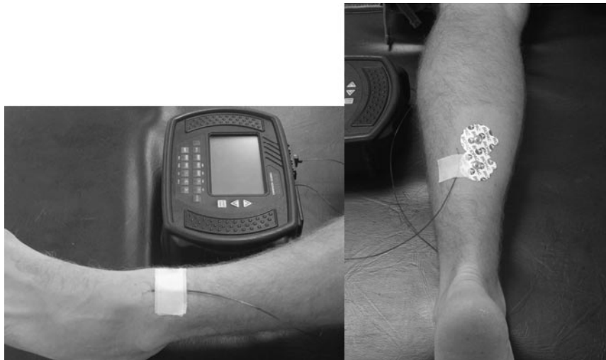
Placement of the surface thermocouples on the ankle (left) and on the soleus muscle (right).
