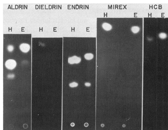
FIGURE 5. Autoradiographs of extracts from excreta (E) and body homogenates (H) of salt marsh caterpillars fed radiolabeled organochlorine pesticides.
