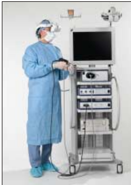
Figure 1. The EndoSite 3Di Digital Vision System (Viking Systems, La Jolla, CA) couples a 3D view with an ergonomic head-mounted display.
