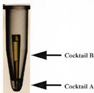
Figure 1. Simple and reliable device compartmentalizing an Eppendorf tube that allows capture, reverse transcription and nested-PCR in a single closed tube. Cocktail A corresponding to the reverse transcription and first PCR reaction mix is added to the bottom of the tube. Cocktail B, the PCR reaction mix for the second amplification, is added into the pipette tip cone.
