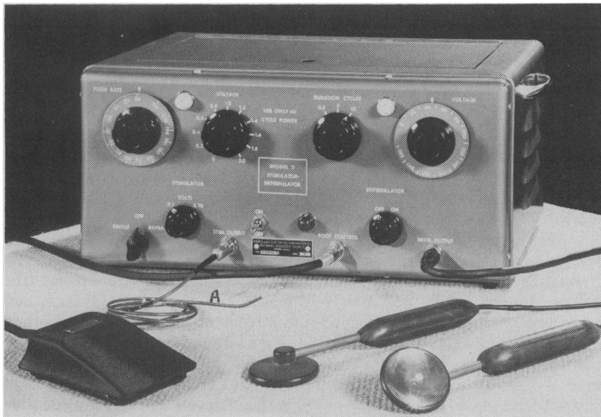
The combined stimulator-defibrillator, with a foot pedal to trip the single 200-volt defibrillating shock. Special electrodes were held on either side of the heart to conduct the electric current through the organ, and (A) an intravenous catheter electrode connected to the pacemaker.
