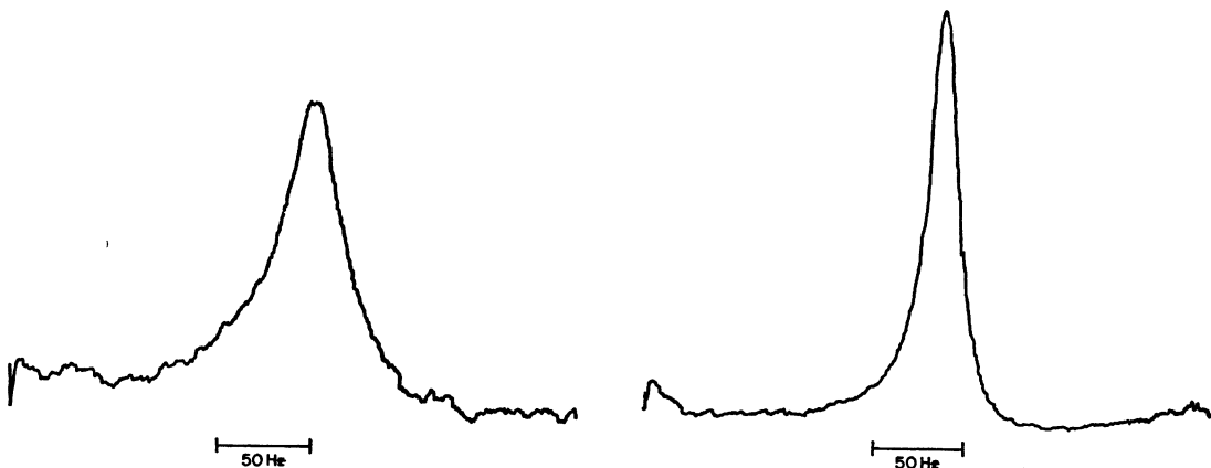
FIGURE 1 NMR sodium signal from whole frog muscle. Left: intact, fresh muscle. Right: signal from same muscle after it had been ashed and the residue dissolved in 0.1 N HCl. The gain sensitivity was one-half that for the intact muscle spectrum.
