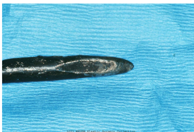
Figure 1. Handle of screwdriver (a) and screwdriver tip (b) used by electrician described in text. Note that fingerprint melted into the handle and that the tip of the screwdriver has been rounded.
