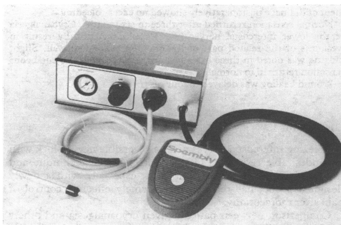
FIG 1—BMS40 console and probe for cryoanalgesia after thoracotomy (Spembly Ltd, Andover, England).
