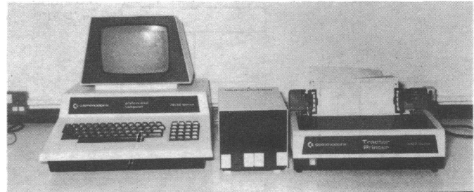
FIG 1—Computer is linked to “floppy” disc unit, which stores programs and case histories. Optionally, the material may be printed out through the interfaced printer.
