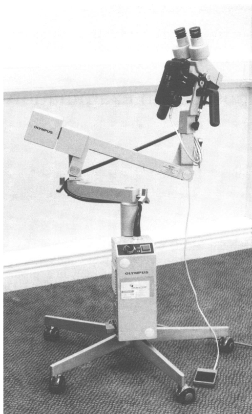
Figure 1 An Olympus colposcope. The instrument is mounted on five radiating legs fitted with castors for mobility. The light source is mounted on the central pillar and light transmitted to the head by fiberoptic cable. The binocular viewing head is mounted at the end of a counterweighted cantilever arm and is shown here with self winding 35 mm single lens reflex camera body attached, operated by remote foot switch. Focal distance from the front of the lens system to perineum is 30 cm with extension lens fitted. Variable magnification is controlled by rotating the small silver wheel above the control handle on the head (range \times 7 to \times 23 ). The arm system can be fixed by tightening the Y shaped bolts.
