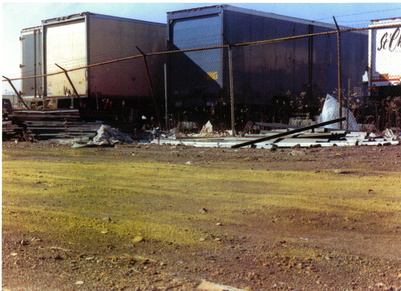
FIGURE 1. Chromite ore processing residue waste site number 2, November 21, 1989. Yellow “chromate blooms” appear at the most heavily contaminated sites. They are most likely to be observed during the dry weather a few days after a rain.
