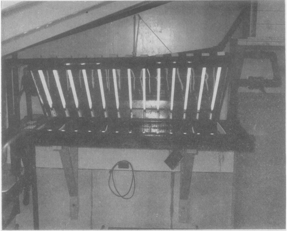
Figure 2—Purdy Ultraviolet Treatment Unit
