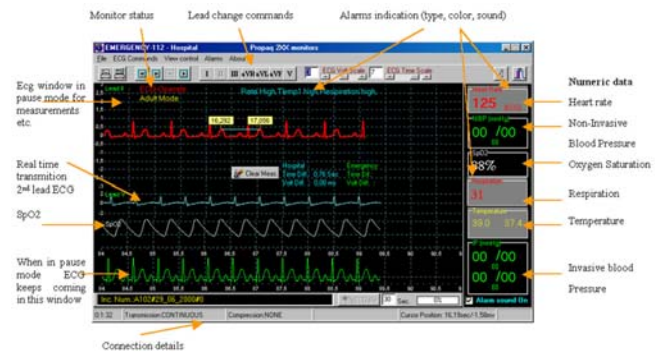
Figure 6 Biosignal receiving window at Base Unit
