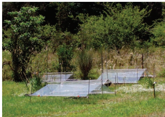
Figure 1. Detail of a field site showing spectral filters used to manipulate the UV environment of plants grown under natural conditions. The site is in the natural area of distribution of N. longiflora , near Huerta Grande (Córdoba, Central Argentina). UV-B absorbing and UV-B transparent filters are shown. Because the UV-B absorbing filters selectively attenuate solar UV-B with minimal effects on PAR, phytochrome-absorbable radiation or total energy balance, the setup is ideally suited to detect highly specific effects of solar UV-B radiation.
