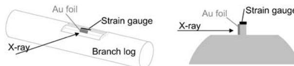
FIGURE 1 Schematic diagrams of sample preparation for the synchrotron x-ray experiment. Three-dimensional view (left) and its cross-sectional view (right).
