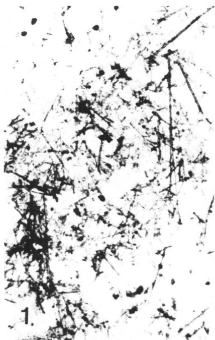
FIGURE 1. Autoradiograph of UICC crocidolite after adsorbance of ^3\text{H} -BaP. When suspended in serumless medium before addition to cultures, fibers are beaded with label. \times 480 .
