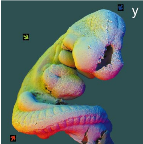
Fig. 6 panel y: 90° sectors of annular solid-state BSE detector, to demonstrate that methods also work for conventionally prepared biological soft tissue SEM samples. 30 kV BSE scanning electron micrograph of 9-day post-fertilization mouse embryo, fixed in 3% glutaraldehyde in 0.2 M cacodylate buffer, post-fixed in 3% osmium tetroxide in same buffer, both for 16 h, dehydrated in ethanol, substituted with Freon-113 and critical point dried from carbon dioxide, mounted on spherical Aluminium rivet, sputter coated with gold. Fieldwidth = 1.85 mm. WD = 17 mm. Three of 4 angular sectors of an annular detector were used to obtain three different images which were then used to synthesize a colour image: coloured arrows show directions of apparent illumination. R = 1 ↗, G = 2 ↘, B = 3 ↙.
