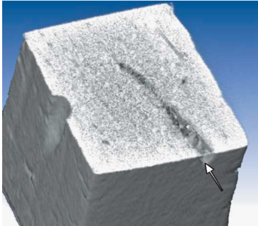
Fig. 7 Micro-CT of bone specimen of cross-section 2 mm × 2 mm. Scratch labelled with iodinated contrast agent shown in Fig. 6.
