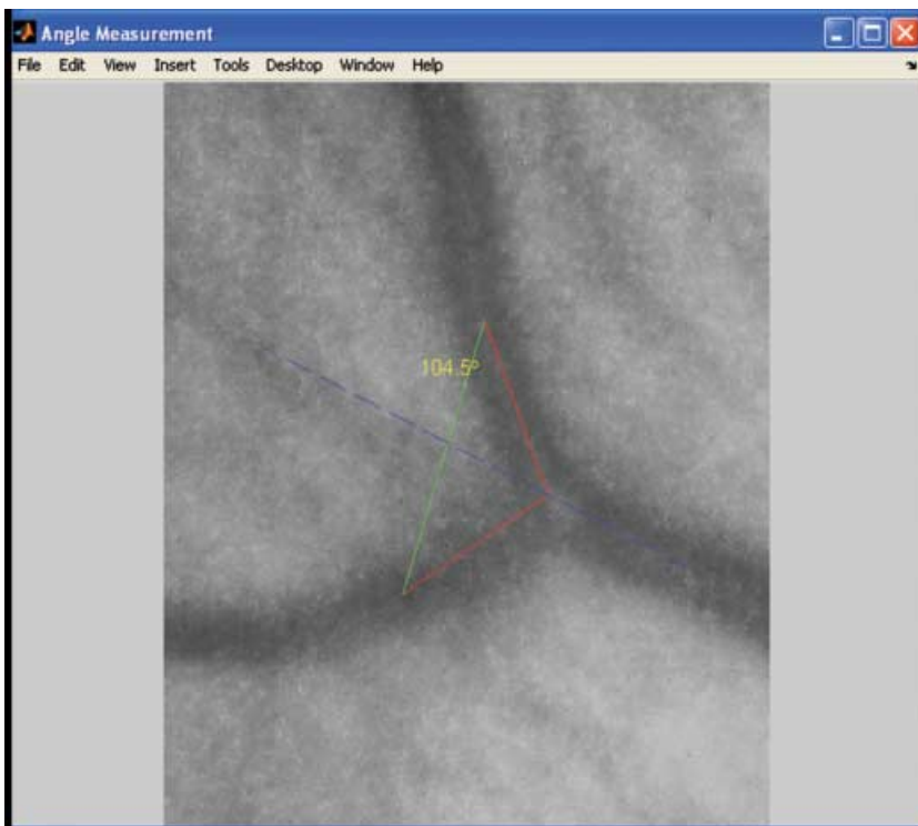
Fig. 7 A region of interest within an enhanced greyscale fundal image has been selected to include a bifurcation of a parent vessel into two daughter vessels. Image analysis programming allows the angle between the two daughter vessels to be calculated.
