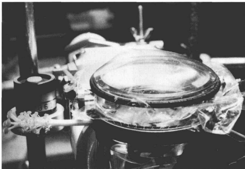
Figure 2. Arrangement for measuring ovarian gas exchange during stimulation of the stigma with pollen, cold shock, and wounding. CO 2 concentration was measured in parts per million with a porometer (Walz CQP-130) at 25°C and a RH of 60%. After the flower leaves were cut off, only the ovary was enclosed by the measuring chamber.
