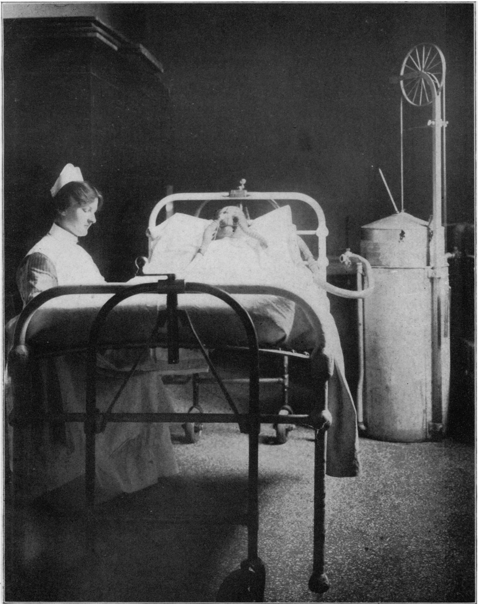
Fig. 2—"RESPIRATORY-VALVE AND SPIROMETER" APPARATUS FOR DETERMINATION OF BASAL METABOLISM AS IN USE AT THE ROYAL VICTORIA HOSPITAL, MONTREAL.—(TECHNIQUE OF DR. WALTER M. BOOTHBY, APPLIED BY M. E. ABBOTT).
