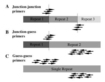
FIGURE 1.—Types of markers tested. (A) Junction–junction primers that flank repeat junctions were most effective, yielding usable markers with 10.3% of the primer pairs tried. (B) Junction–guess primers and (C) guess–guess primers were much less effective, yielding a 0.4% success rate. At least three primers were designed for each end of all amplicons.
