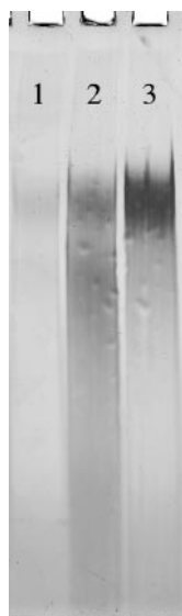
FIG. 5. Analysis of LTA isolated from L. brevis TMW 1.465 and L. brevis TMW 1.465A: electrophoretic separation of cdLTA purified from L. brevis TMW 1.465 grown under reference conditions (lane 1) or acid stress conditions (lane 2) and from hop-adapted L. brevis TMW 1.465A (lane 3). The samples loaded represented equivalent cell dry masses for the different conditions, and the results are representative of two independent LTA isolations.
