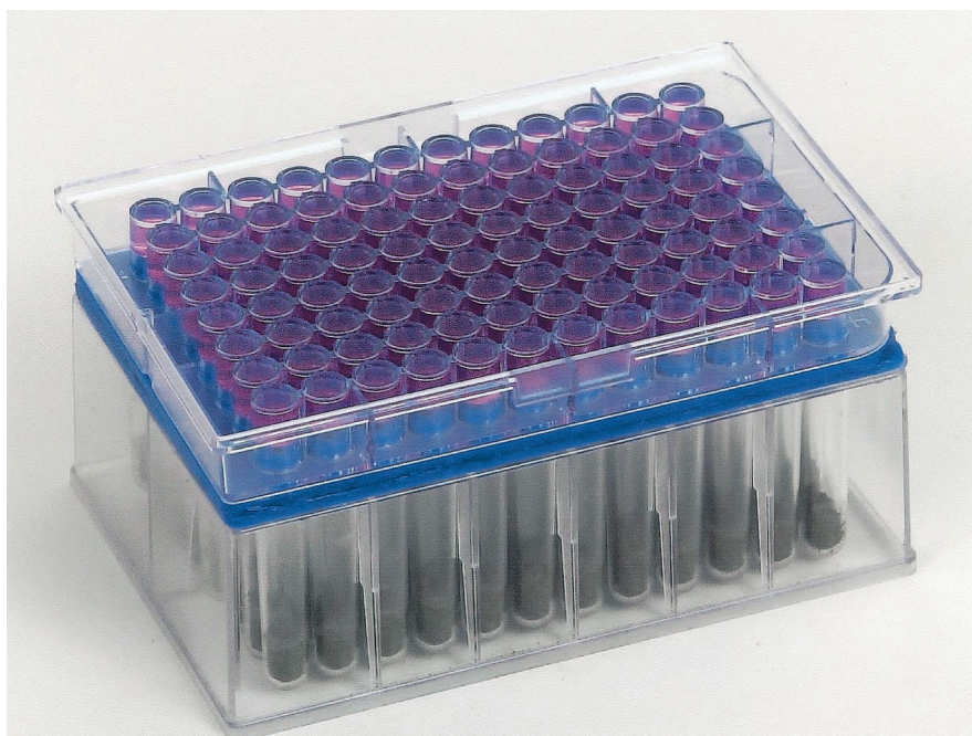
FIG. 2. Assembled MicroResp system comprising a deep-well microtiter plate to hold soil, an interconnecting gasket, and a top plate with a detection gel.
