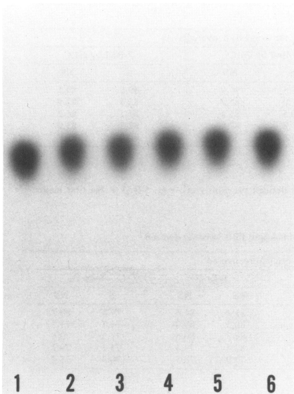
FIGURE 1. Autoradiogram of TLC plate showing ^{14}\text{C} -PBB standard and ^{14}\text{C} in extracts after incubation in soil: (1, 6) ^{14}\text{C} -PBB standard; (2, 3) extracts from sterilized soil after 6 and 12 months incubation, respectively; (4, 5) extracts from nonsterilized soil after 6 and 12 months incubation, respectively.
