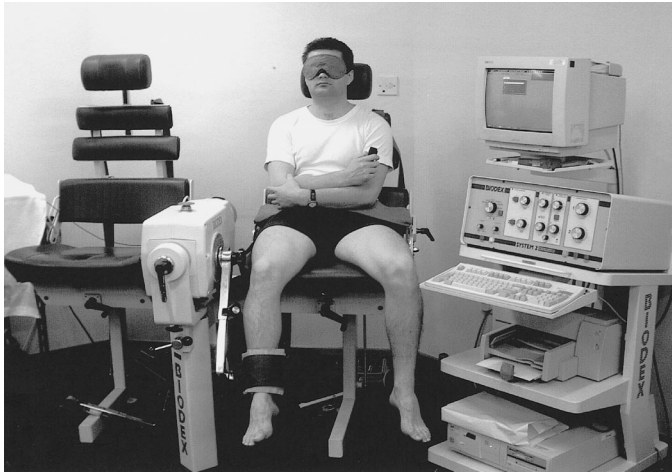
Figure 1. Patient setup on the Biodex dynamometer.
