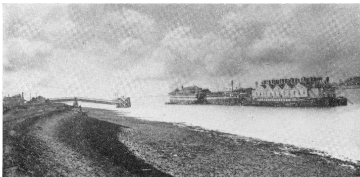
Fig 1 General view of the ships Atlas , Endymion and Castalia (nearest the camera), together with dummy pier, and laundry on shore. Note the double hull of the Castalia
